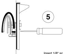
Insert 1/8" screwdriver in the steering slot below the lens. Using the screwdriver, bend the mount to point the camera in the desired direction. Never use the camera to bend the mount!
